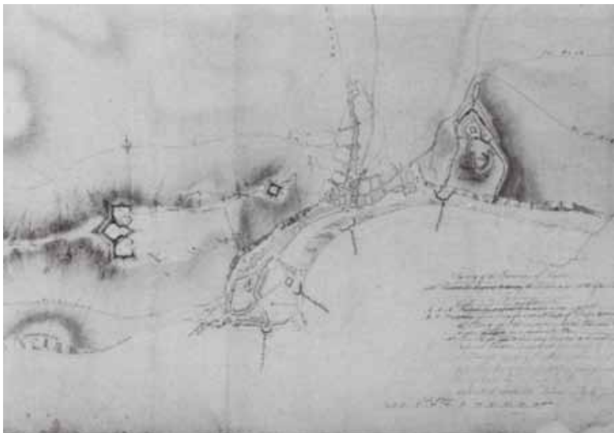
Plan showing the proposed defensive works on the Western Heights, with annotations showing their fields of fire; undated, but probably 1780-1 and before 1784; unsigned, but probably drawn by Lieutenant Thomas Hyde Page (KA Do P/1)
