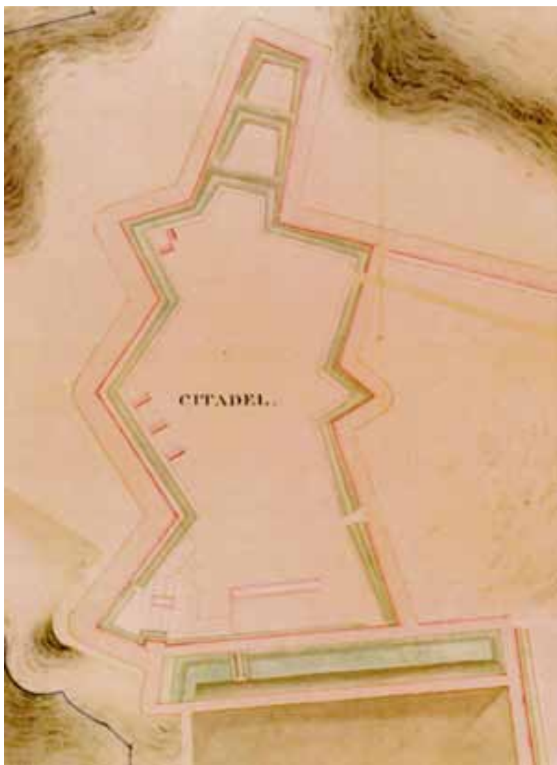
Plan of the Citadel, showing five expense magazines on the western side, drawn 1830 (extract of NA: WO 55/2562/8)
