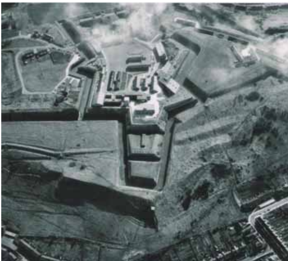
The inclined steps (killing zones) west and east of the Citadel’s North-West Bastion, photo taken 1978
