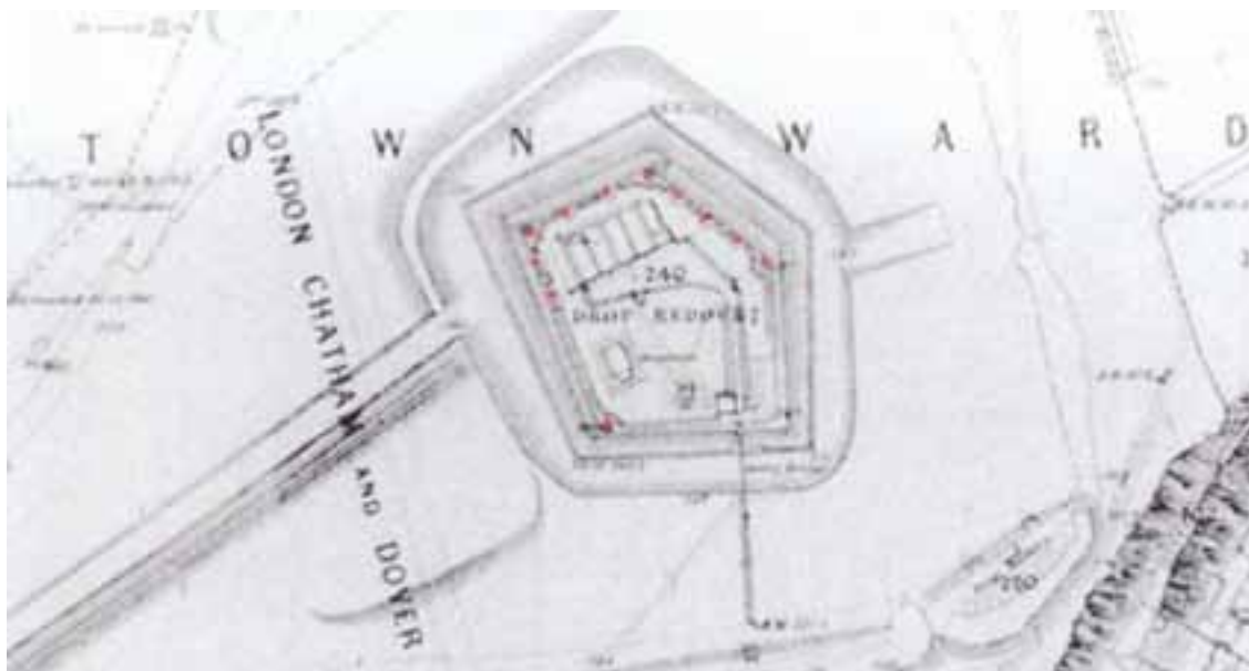
Plan of the Drop Redoubt, drawn c. 1860 (NA: WO 78/2555/10); gun positions on the terre-plein were highlighted in red by RCHME Report No. 3: Figure 14b
