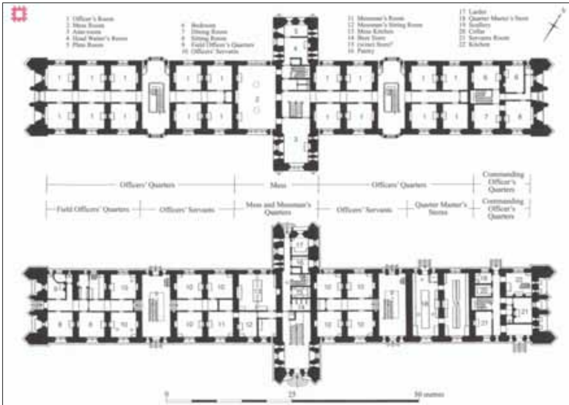
The Officers' Quarters in the Citadel, plan of the ground floor (lower drawing) and first floor (upper drawing) (after HMPS: 402584; RCHME Report No. 2: Figure 65)
