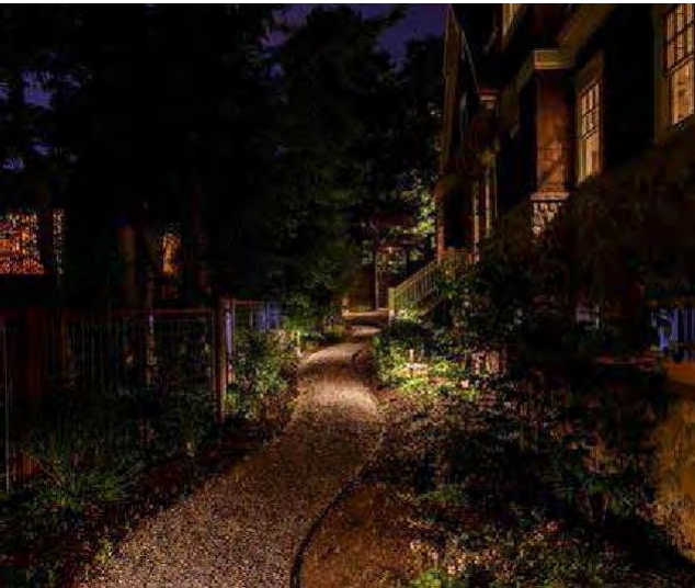
Figure 64: Example of path lighting where all lights are directed
