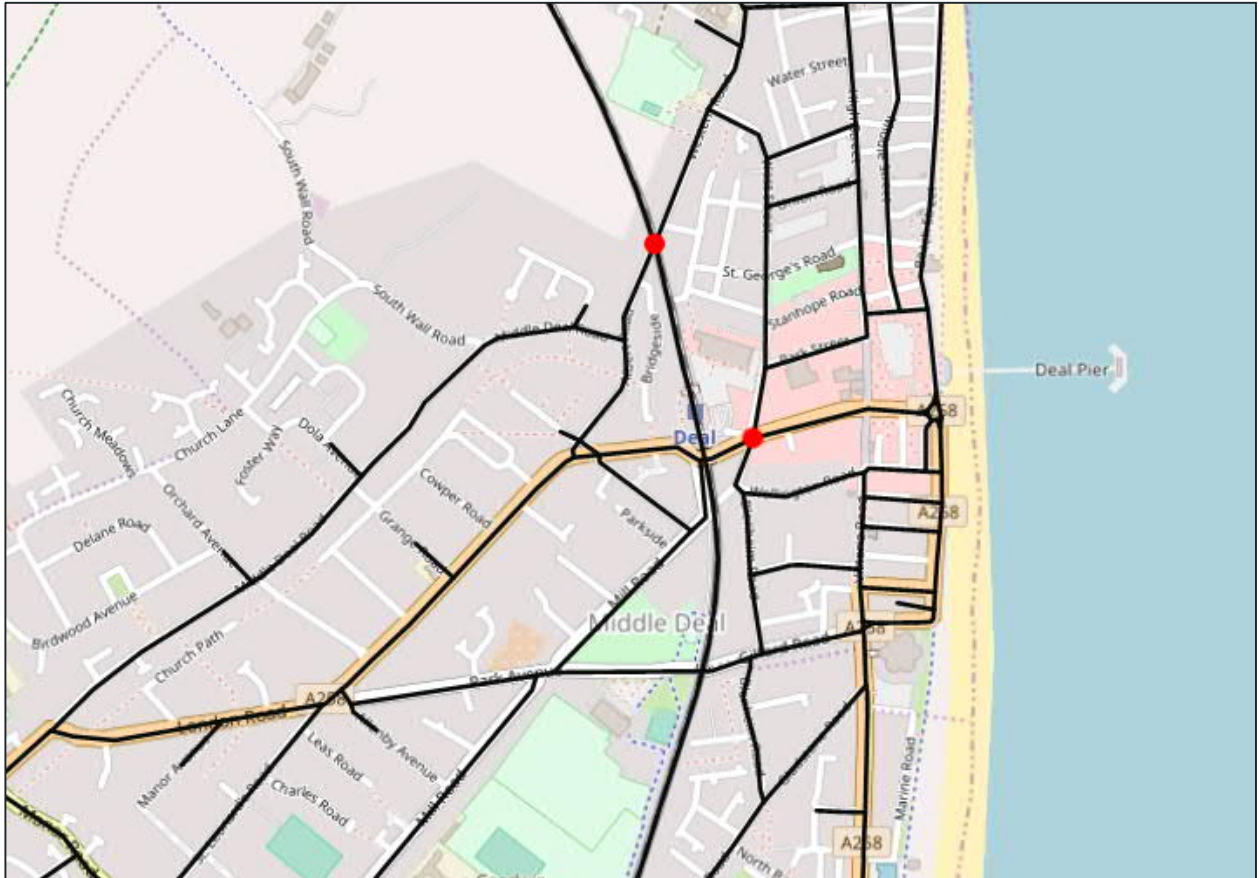
Figure 2: Signalised Junctions in Deal Area
