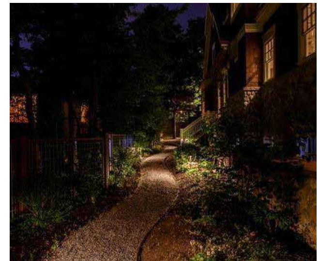
Figure 73: Example of path lighting where all lights are directed downwards, while the light sources are obscured, elsewhere in the UK.
