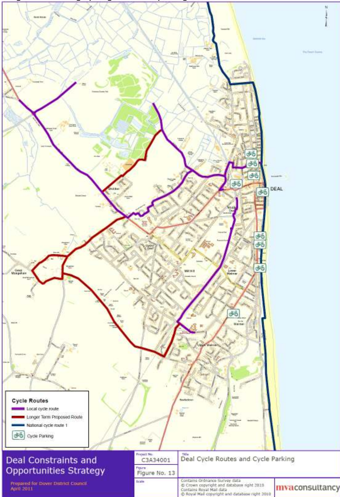
Figure 41 - Existing cycling routes and parking
