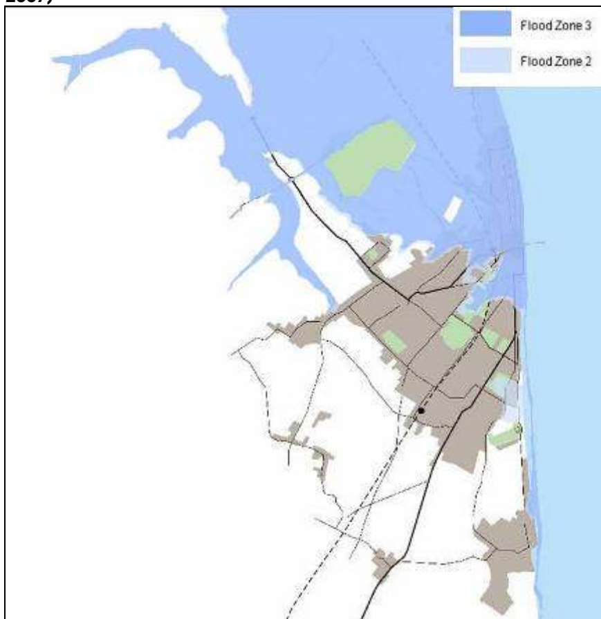
Figure 13: Flood zone map without considering the existing flood defences (Source: SFRA 2007)
