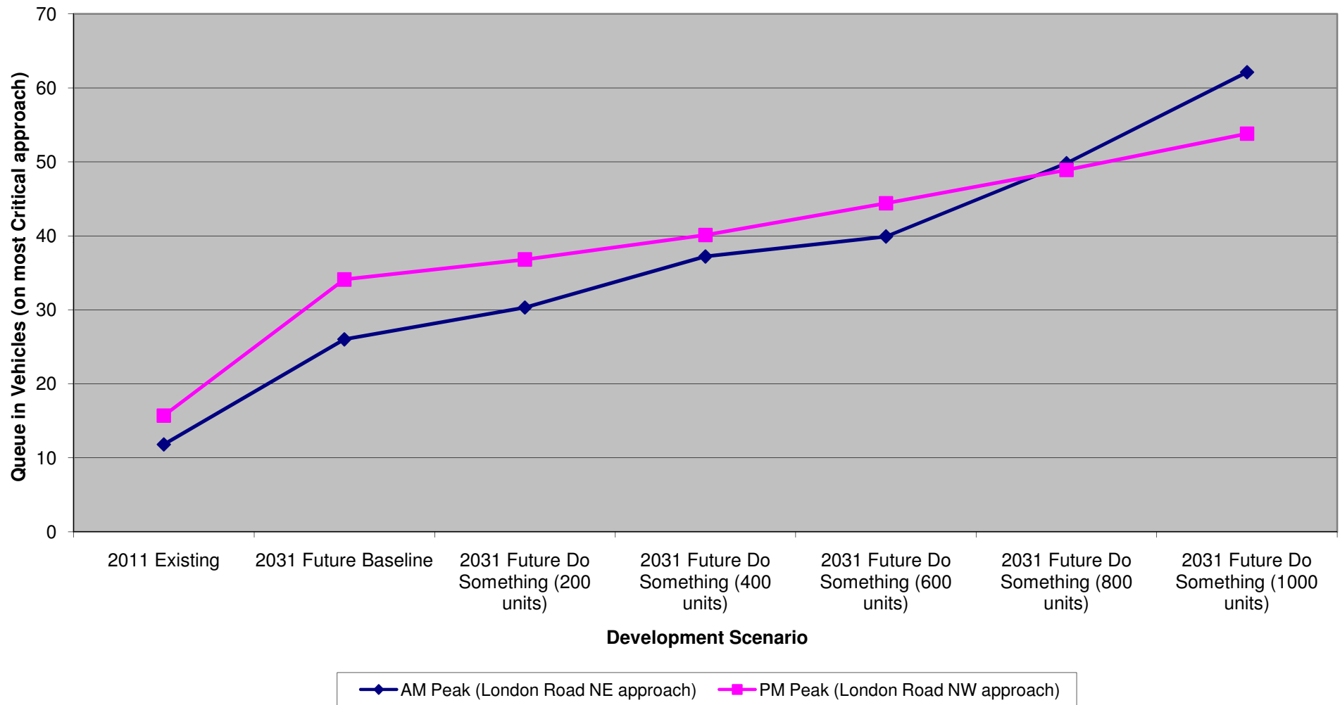
Figure 4.7: A258 London Road / Manor Road (Option 2 - Signal Controlled Junction with right turn ban from Manor Road)
