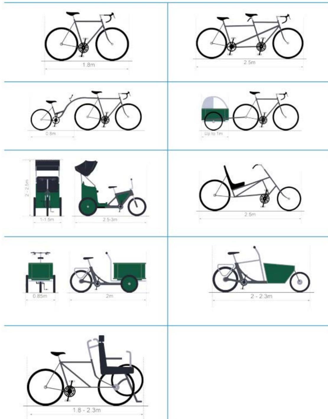
Table 5-1: Size and minimum turning circles of cycles
