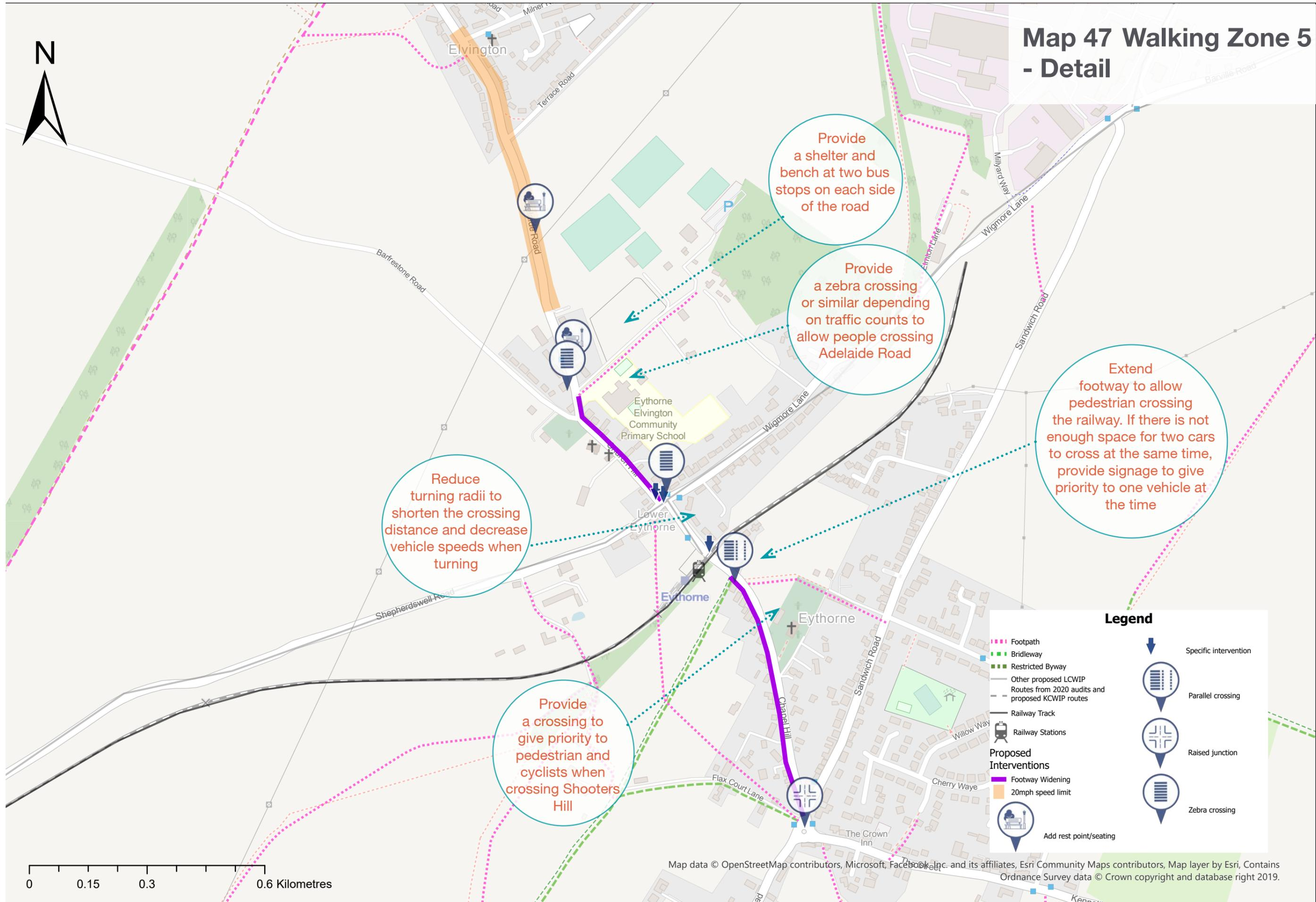
Reduce turning radii to shorten the crossing distance and decrease vehicle speeds when turning
