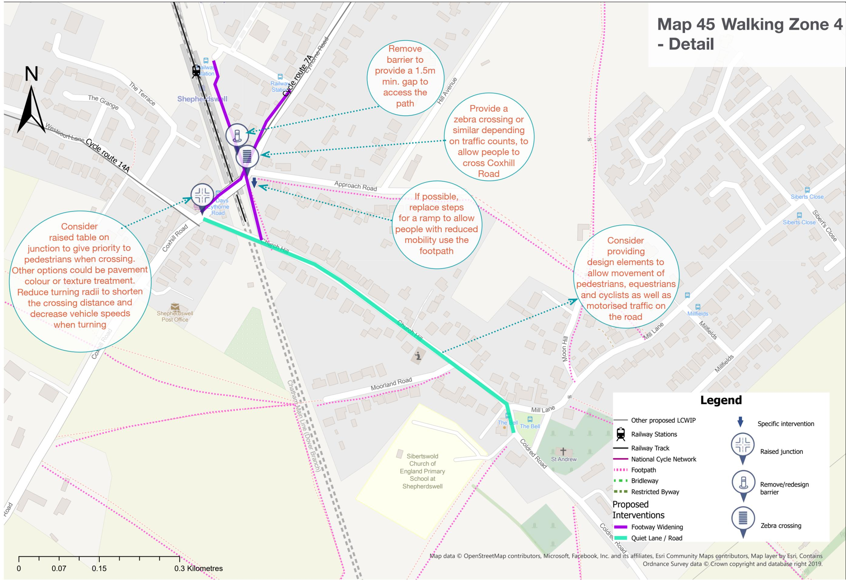
Consider raised table on junction to give priority to pedestrians when crossing. Other options could be pavement colour or texture treatment. Reduce turning radii to shorten the crossing distance and decrease vehicle speeds when turning
