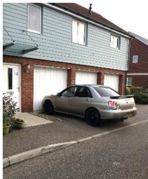
Left - Example of a double open car port. Above - An example of poor design, resulting in footway obstruction due to an overhanging parked vehicle.
